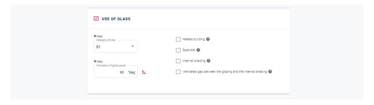
To ensure a safe design, tick the relevant checkboxes on the right. For example, spandrel glazing can typically become very hot, which needs to be noted.
