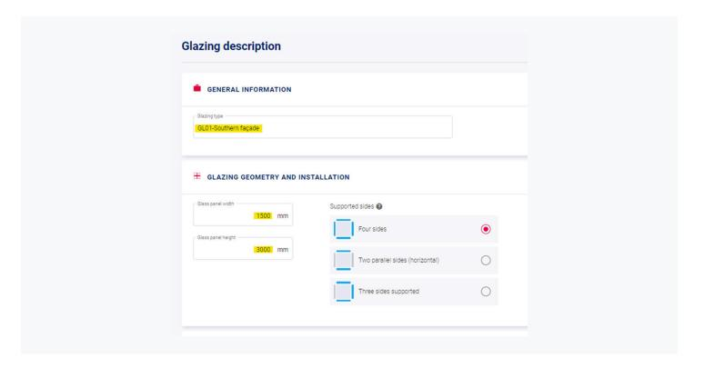
Next, the type of use defines the function of the room adjacent to the installed glass: **Office**, **Home**, etc. For vertically installed glazing, the installation angle should remain set at 90°. The **Use of Glass** parameter is important for evaluating the correct temperature in the insulated glazing units.
